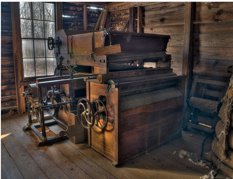
Cotton Gin. The gin processed roughly one bale (500 pounds on average) per hour. Credit: Jarrell Plantation.
